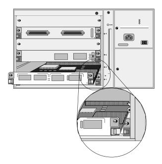
Figure 3-5. Installing the 7F06-02 Module in the 7C04-R Workgroup SmartSwitch
